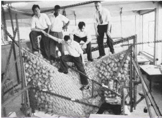
) calculations and scale models were tested, concluding that the skin should be constructed with a 5-centimeter-thick prestressed concrete shell
